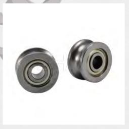
Package contains: 1 x U-groove bearing 624ZZ U-groove bearing 624ZZ. Inner diameter: 4 mm Outer diameter: 13 mm Thickness: 4 mm Single row deep groove ball bearing. Has 2 metal covers to prevent dirt from affecting the balls. The bearings are pre-lubricated.
